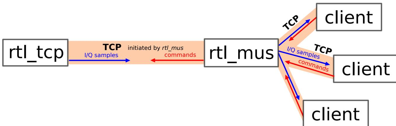
*rtl\_mus* will allow multiple clients to connect to your I/Q source simultaneously, and control its parameters.
