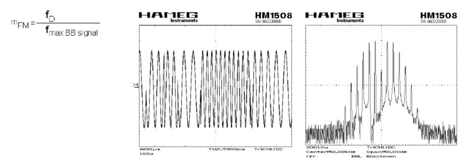
Bandwidth: infinite (in principle, as described by Bessel functions), in practice approximated as
