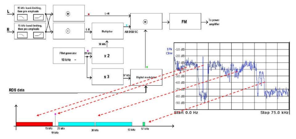
And the stereo transmission, pilot signal and RDS (and SCA, if applicable)
