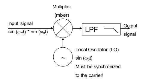
Demodulation of a DSB / SC signal:
