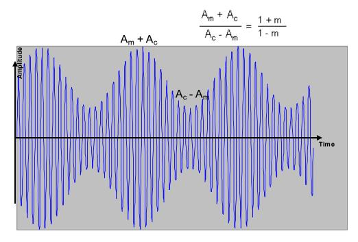
If x (t) =  $A_m * \sin(\omega_m t)$  and the carrier's amplitude is  $A_c$ , then:
